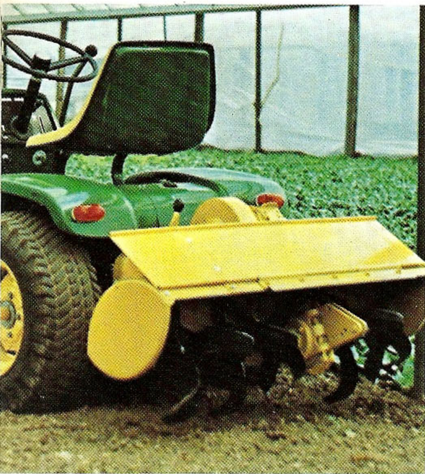
Working width for the "140" tiller goes to 42 inches.
