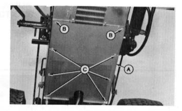
20. Install screen (A) and fasten it with two no. 10 screws and washers (B) from kit and screws (C) removed in Step 4.
