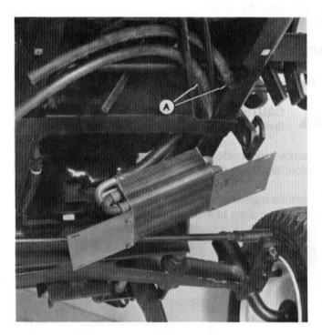
16. Install hoses and conduit (A) through hole in firewall.
