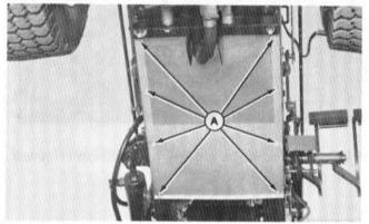
4. Remove bottom screen by removing bolts (A).
