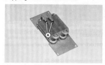
7. Remove plugs (A) in oil cooler.
