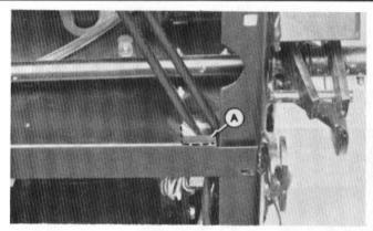
Tractor with serial number M479450 and below: Cut hole (A) in right side of firewall as shown.
