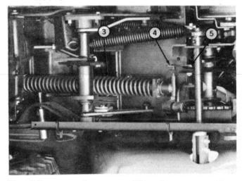
Place spring assembly above secondary lift shaft as shown above.
