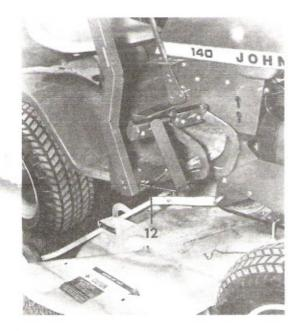
Bolt pedal guard to right support bracket using ¼" x ¾" hex head bolts and nuts.
