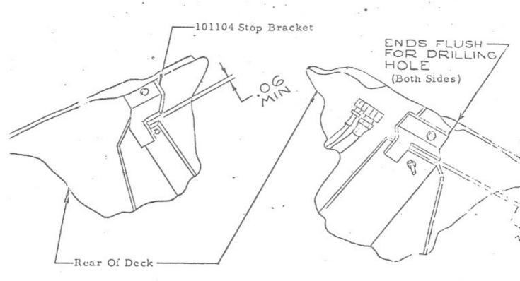
Template For Drilling Holes in Left Hand Step to Install Part No. TY 2033 on JOHN DEERE 140 Lawn & Garden Tractor
