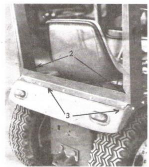
Set rear upright up on fenders to see that marks on fender line up with 2 inside holes.
